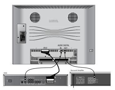
Connect the output socket of the DVD player (DIG OUT) to the TV's "AUDIO DIGITAL IN" socket with a cinch cable.
